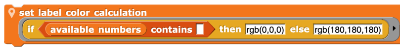
Figure 21: Setting a color calculation. In this example, numbers that the user generates are printed black; others in gray.
